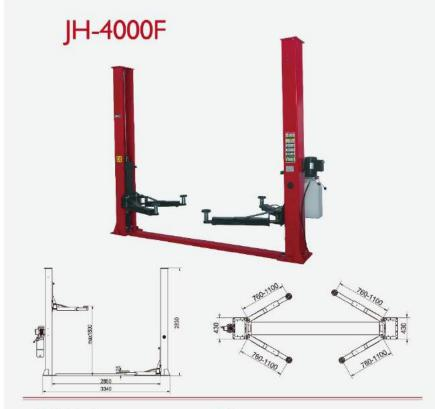
Lifting capacity:4000kgs Lifting height:1800mm Min.height:125mm Overall height:2830mm Overall width:3340mm Width between posts:2850mm
