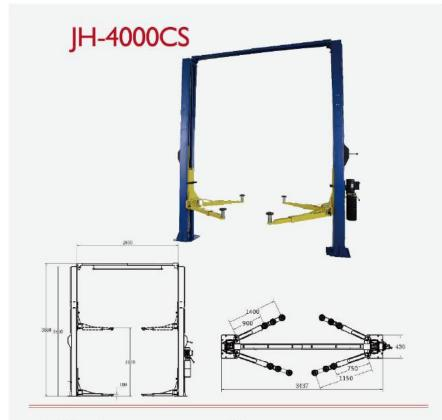
Lifting capacity:4000kgs Lifting height:1800mm Min.height:100mm Overall height:3880mm Overall width:3437mm
